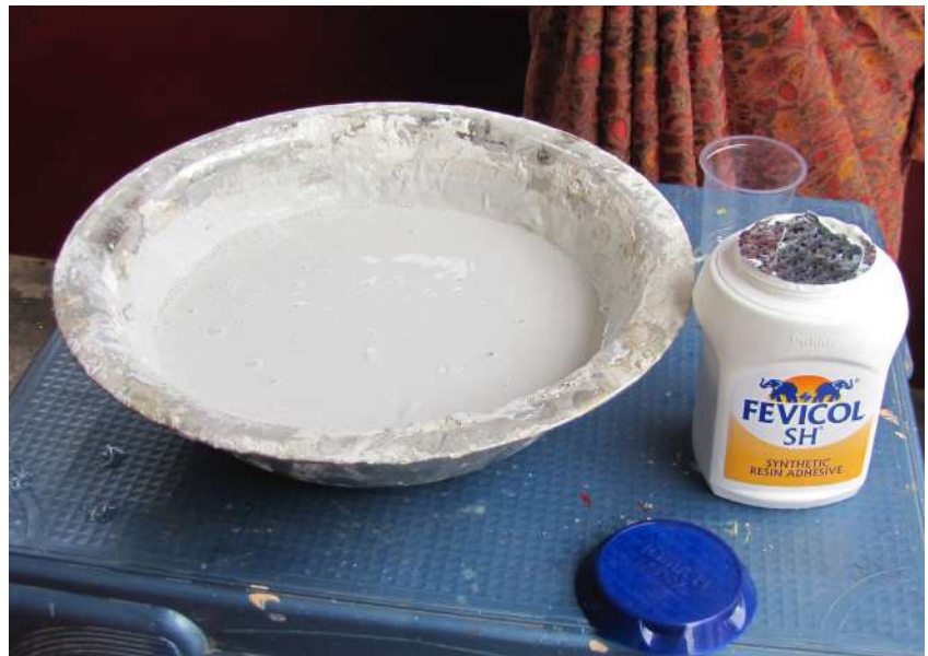
The ready solution used for coating the wrapped structures
