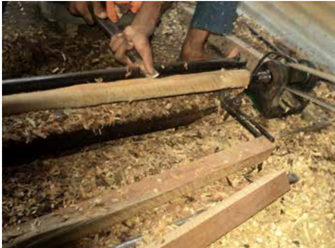
Character Toy 1 - stick turning on Lathe
