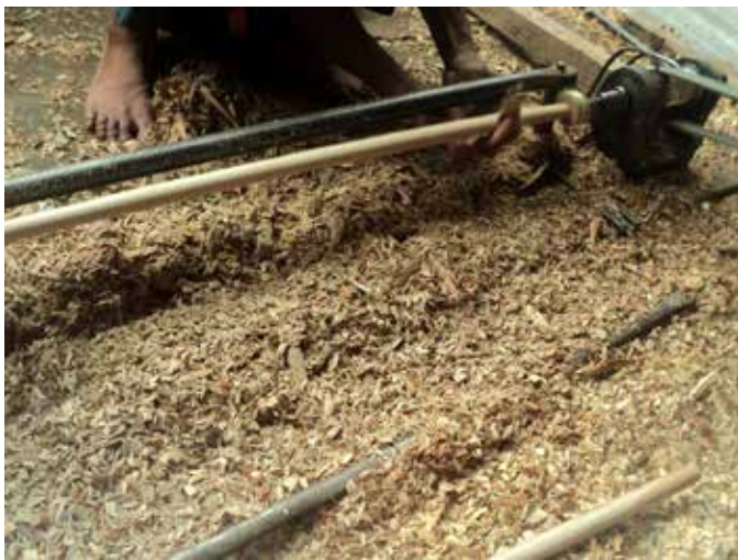
Character Toy 1 - stick sanding on Lathe
