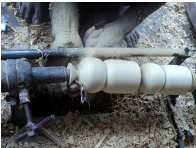
Character Toy 1 - sanding on Lathe
