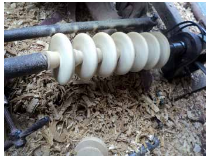
Character Toy 1 - wheels sanding on Lathe
