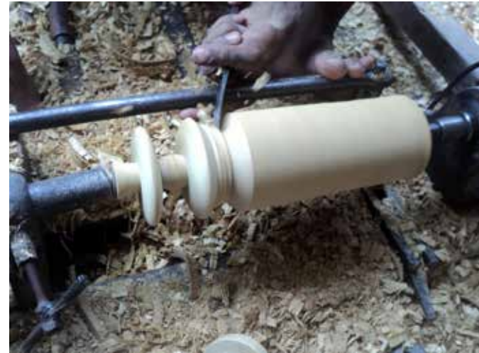
Character Toy 1 - wheels cutting on Lathe
