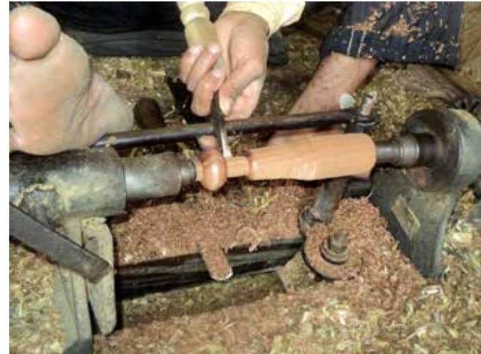
Character Toy 1 - hand cutting on Lathe
