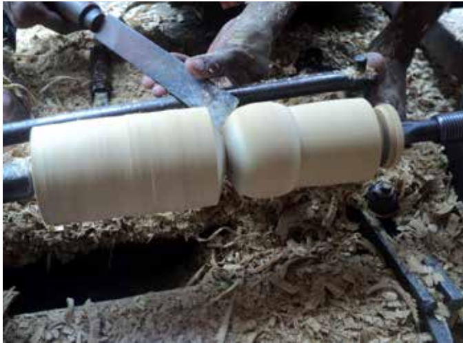
Character Toy 1 - turning on Lathe
