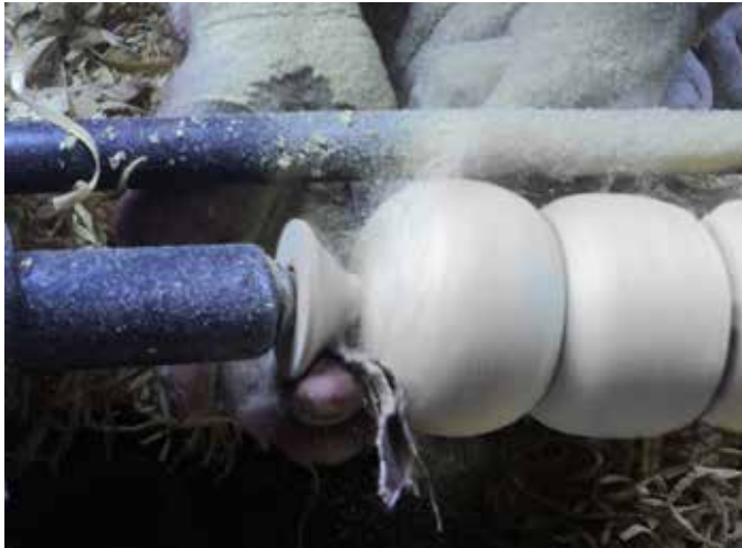
Character Toy 2 - sanding on Lathe
