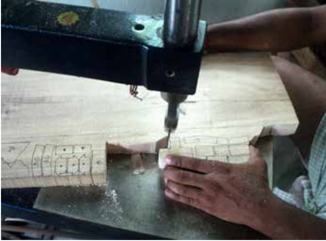
Hill Toy 2 - cutting on Zig Saw
