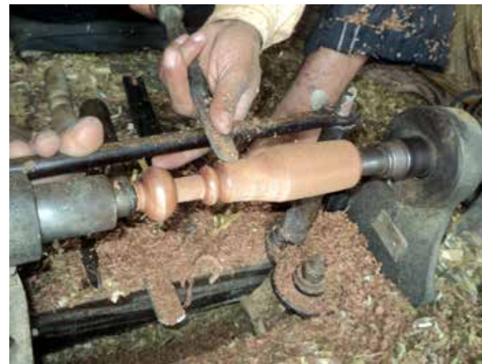
Character Toy 1 - hand finishing on Lathe
